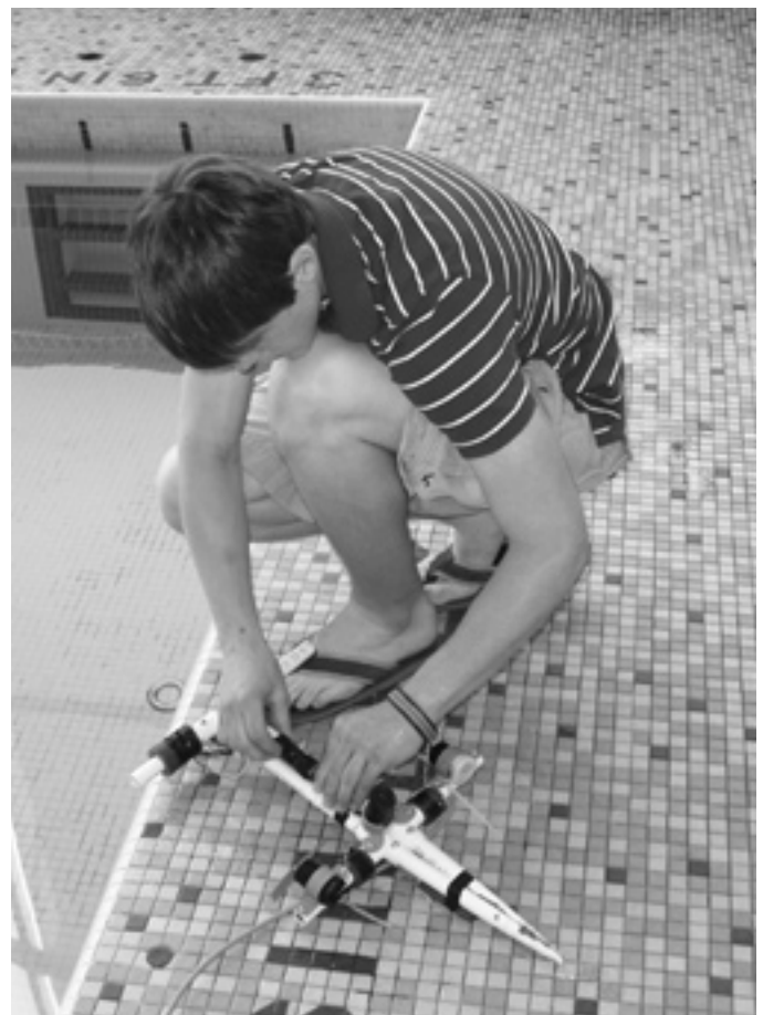
Trevor is adjusting the electromagnet. He is using the extra weight of the electromagnet to make his project neutrally buoyant.
